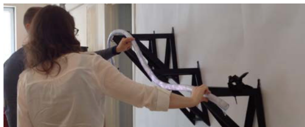
Fig. 5. If the users keep touching for three seconds, the light changes from blue to white, and then expands and shrinks three times to indicate water will come out from the end of the tube.
