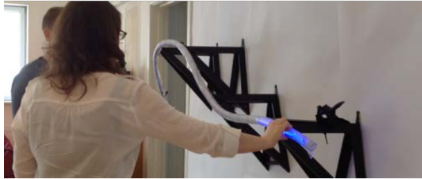
Fig. 3. When a user touches on a single contact point, the blue light moves to the position of the hand.
