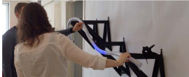
Fig. 4. When users touch two contact points, the blue light moves to the middle position between the points.
