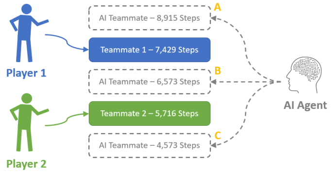
Fig. 1. Two participants teammates remotely engage a software activity each day in which both teammates’ steps from the previous day are presented. A third teammate, not known to the participants to be artificially constructed, is added to the team by the AI. The MAB determines the placement of the AI teammate’s steps relative to the steps of the participants (option A, B, or C), providing additional comparison opportunities that can leverage the SCO preferences modeled for both participants.
