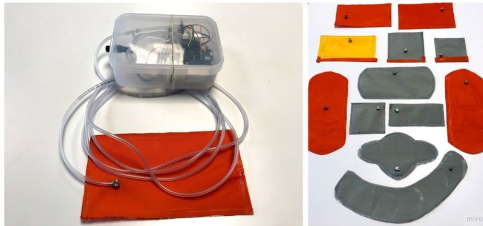
Figure 2. Shape change sensor-actuators, and pillow shapes
