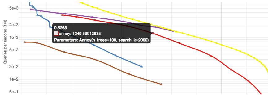
■ Figure 3 Interactive plot screen from framework’s website (cropped). Plot shows “Queries per second” ( y -axis, log-scaled) against “Recall” ( x -axis, not shown). Highlighted data point corresponds to a run of Annoy with parameters as depicted, giving about 1249 queries per second for a recall of about 0.52.
