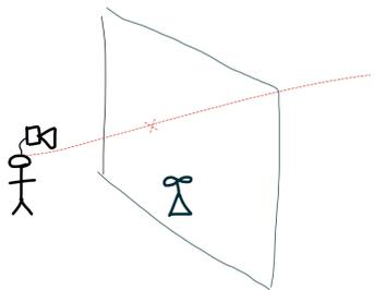
**Figure 8:** This figure shows the same concept of the figure 3 but with a 3D robot (craft) that be moved inside a virtual plane by the gaze. The movement in the third dimension (along the gaze direction) is controlled by looking at the craft and through continues head movements.
