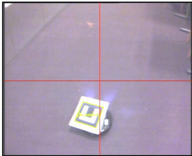
**Figure 1:** Controlling a Roomba vacuum cleaner by gaze in a mobile situation. The user's PoR is shown (cross hair) in the scene image of the mobile gaze tracker in the bottom image.
