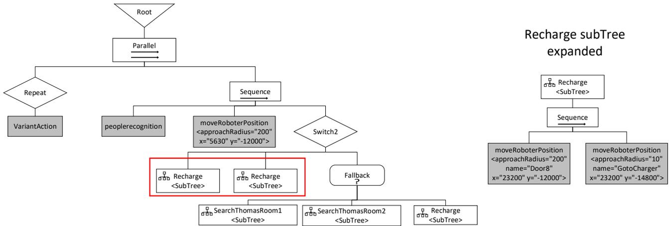
**Figure 4.** Behavior tree model of a retirement home robot from project bundles. The red box highlights an example of a reuse by reference for a sub-tree Recharge (expanded on the right side). A legend is shown in Figure 2.
