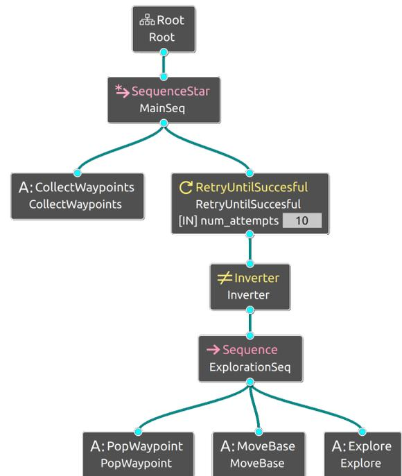
**Figure 1.** An example behavior tree of a health and safety robot inspector from a GitHub project `kmi-robots/hans-ros-supervisor` shown in the Groot editing and animation tool from `BehaviorTree.CPP`
