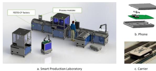
**Fig. 1.** Overview of the Smart Production Lab
